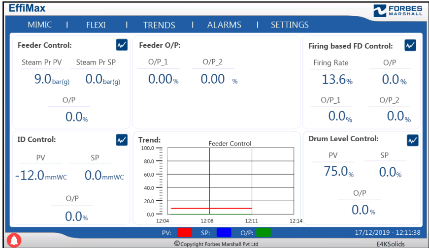
Fig. 2- effiMAX Control System
