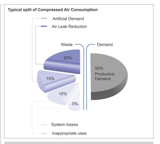
The compressed air demand in plants across industry fluctuates constantly due to intermittent use of pneumatic equipment. This results in low efficiencies and high energy bills. A proper balance between supply and demand of compressed air is essential to control these losses.
