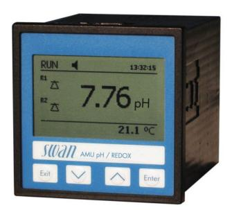
Measuring and control transmitter for panel installation in a Noryl<sup>®</sup> resin enclosure, 96 x 96 x 120 mm (DIN 43700)
